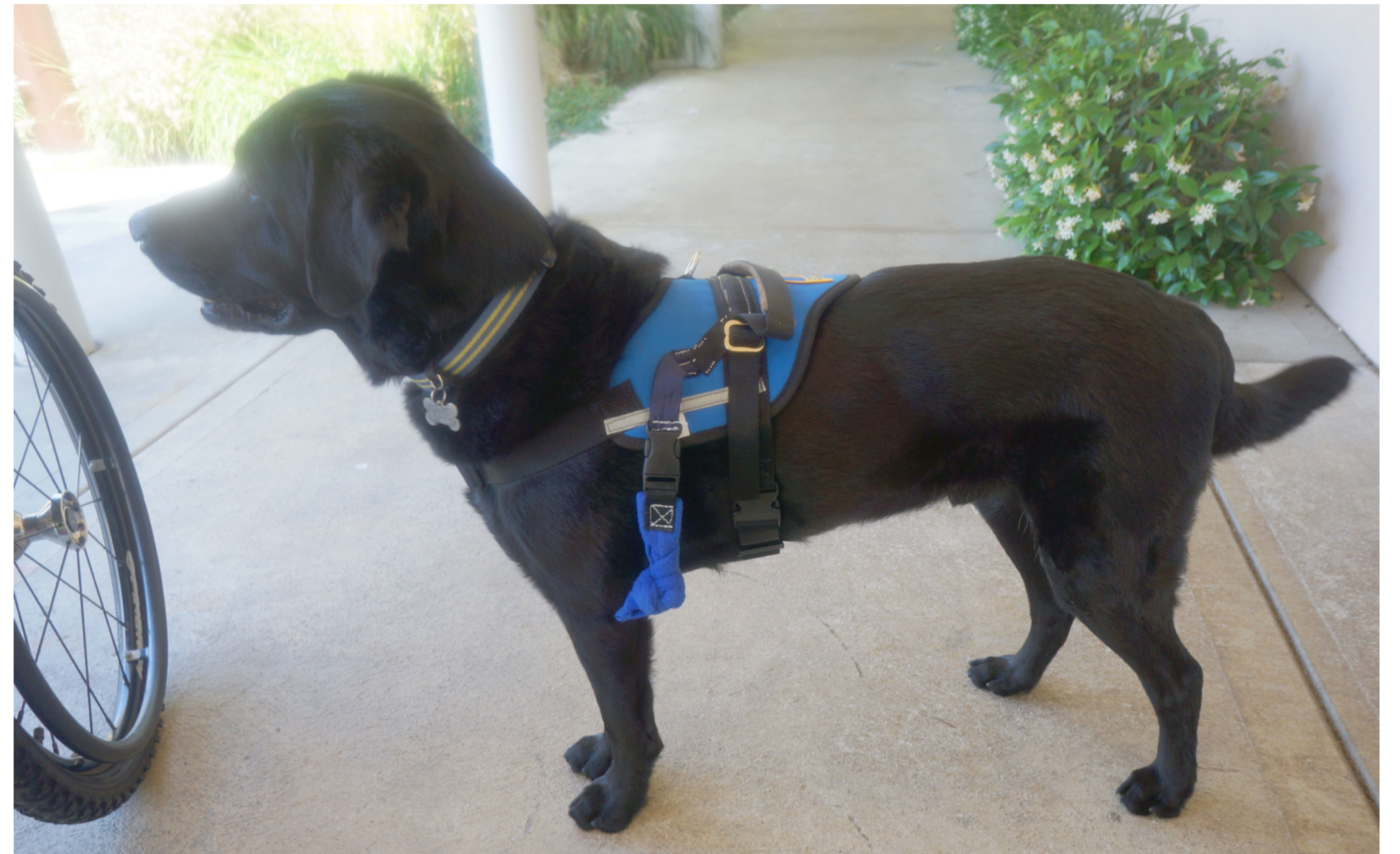
"Call for help" tug sensor for service dog of owner with dystonia.
