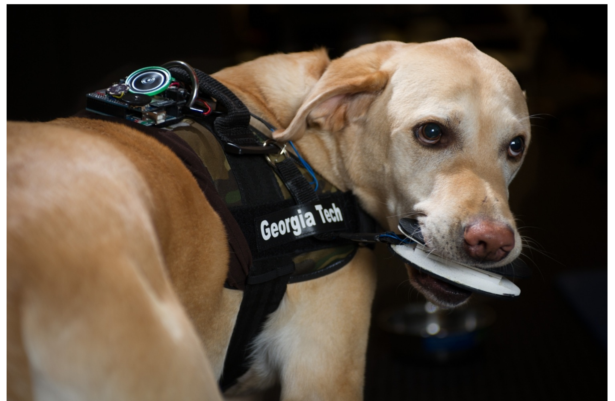
Bite sensor used by guide dog to alert owner of "wait" vs "go around" obstacles.
